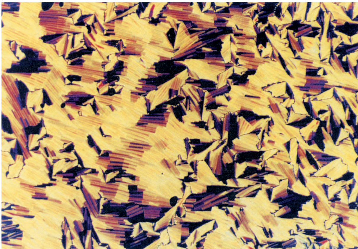
Figure 3. Fan-shaped texture after shearing the mosaic texture of compound 1 (132°C).
