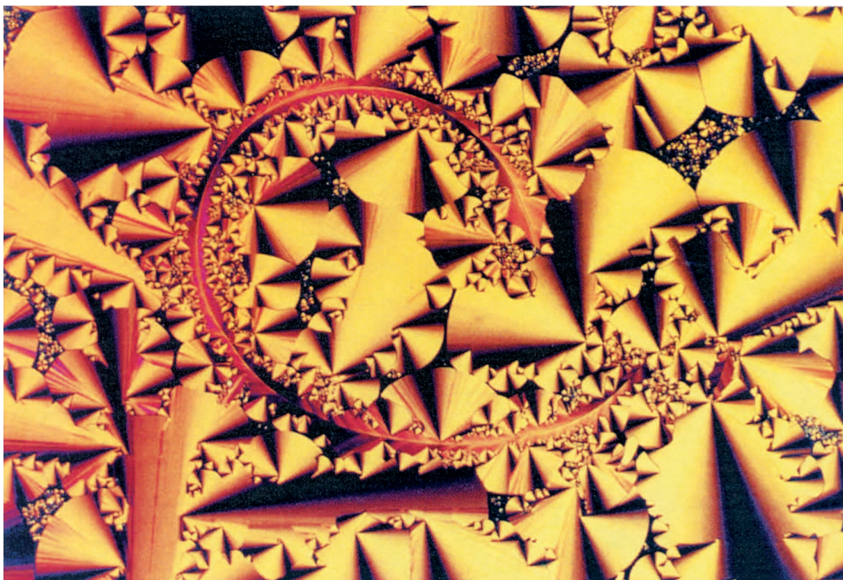
Figure 4. Texture of the B II phase of compound 2 (170°C).
